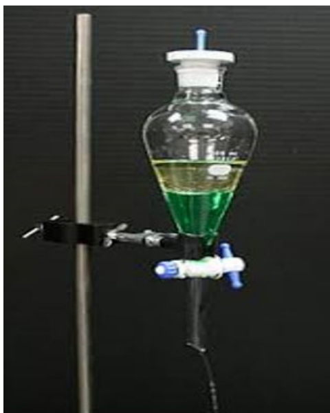
Figure 2: An equilibrium of dissolved substance distributed between a hydrophobic phase and a hydrophilic phase is established in special glassware such as this separatory funnel that allows shaking and sampling.
